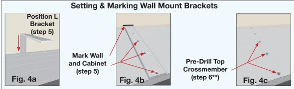
\*\*Note: If ceiling clearance allows, you can drill and fasten the L brackets into the top crossmember in step 7 below, no pre-drilling neccessary.
